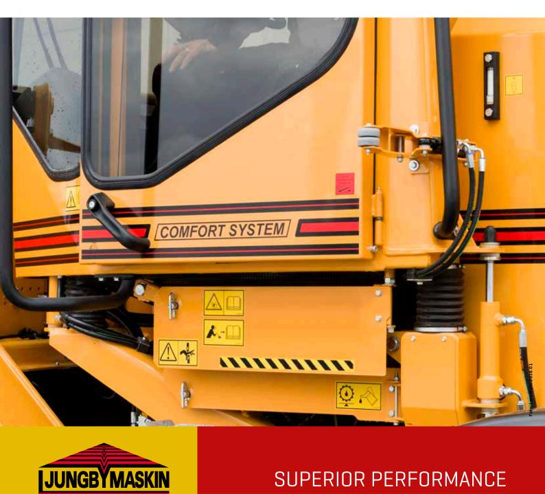
■ WITH A SIMPLE PUSH OF A BUTTON, THE DRIVER CAN CLOSE THE DOOR WITHOUT HAVING TO EXTEND OUT OF THE MACHINE TO REACH IT - A POPULAR AND UNDERRATED TOOL IN OUR QUEST FOR GREATER OPERATOR COMFORT.
